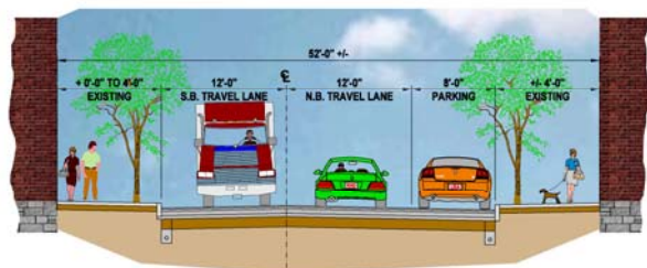
Typical section with single side parking
